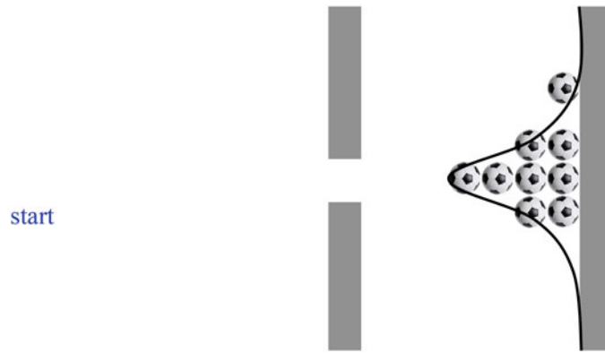
Fig. 3.2 Classical single-slit experiment. Those balls that do make it through the slit form a bell-curve distribution on the far wall.
